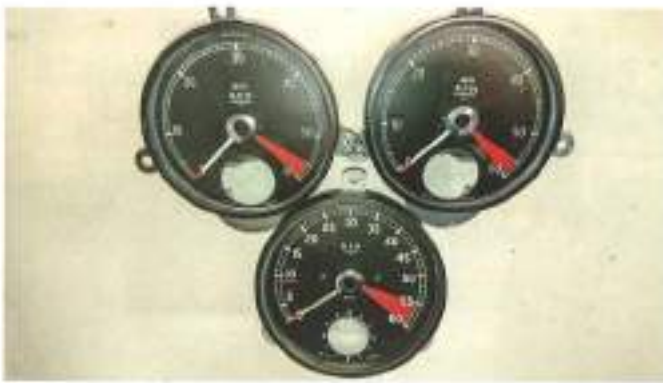
Top l/r early/late mechanical rev counter faces, below electronic – note red arrow at 900rpm and clock markings on face, plus rev numerals at 500rpm as well as 1000rpm increments
