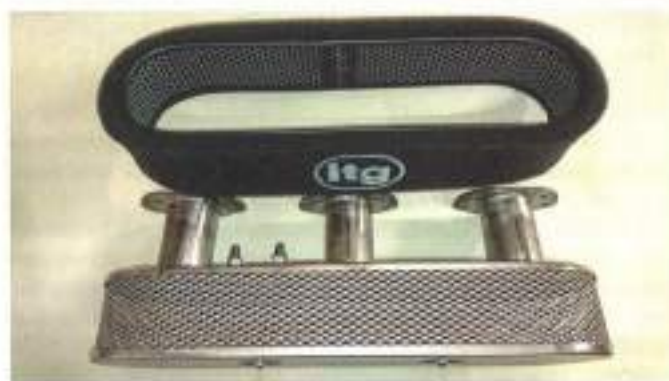
The later 'S' airbox and ITG racing element: lasts for ever, wash in spirits, re-oil and re-fit.
