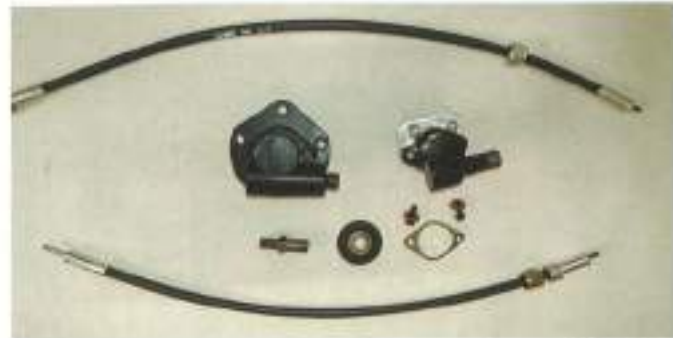
Early rev counter drive equipment; bottom and centre right CAC's conversion from electronic drive to XK manual gauges
